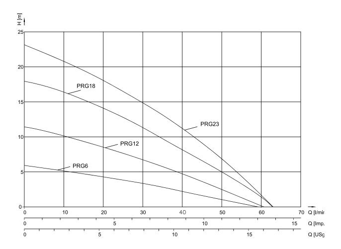
The data apply to fluids with a viscosity of 1  $\rm mm^2/s$  at a density of 1  $\rm kg/dm^3$
