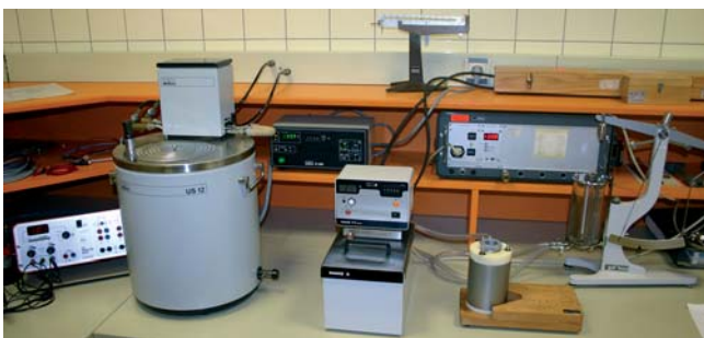
Temperature sensors are calibrated using several test installations
